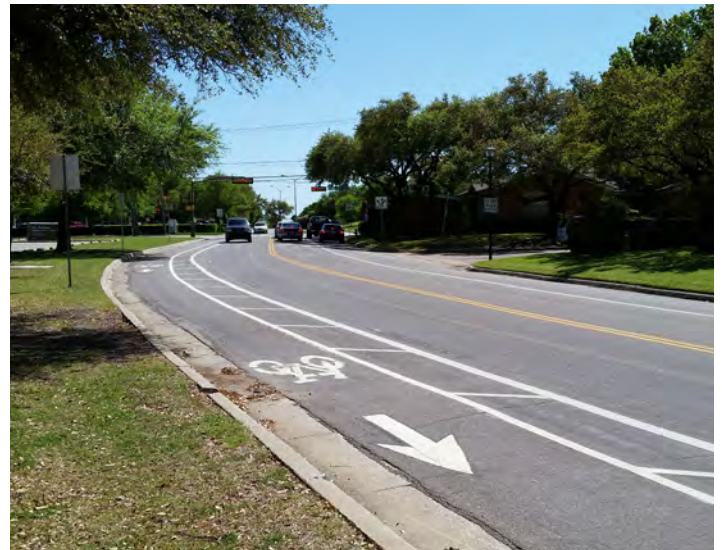
Buffered bike lanes can use paint to increase separation
