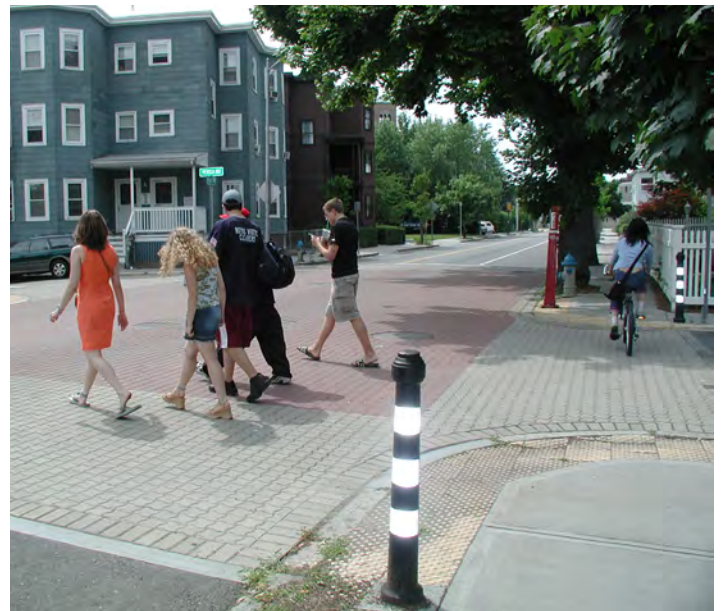
Unique materials for the crosswalk can add to the sense of place along with designating a location for crossing
